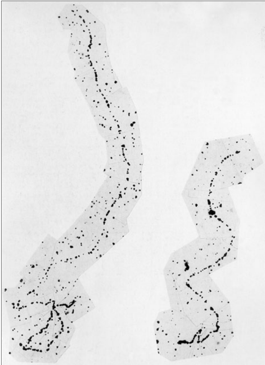
Figure 2.4. Left: Tracks of slow electrons showing the large amounts of multiple scattering that result from the electrons' small mass. Note also the increase in ionization as the electrons slow down. The tracks shown are about 0.2 mm long. Right: Proton tracks (about 0.2 mm long) show a generally much higher degree of ionization and are much straighter, even to the very end where they stop (at the top of the photo). (Photographs courtesy of Peter Fowler, University of Bristol.)
