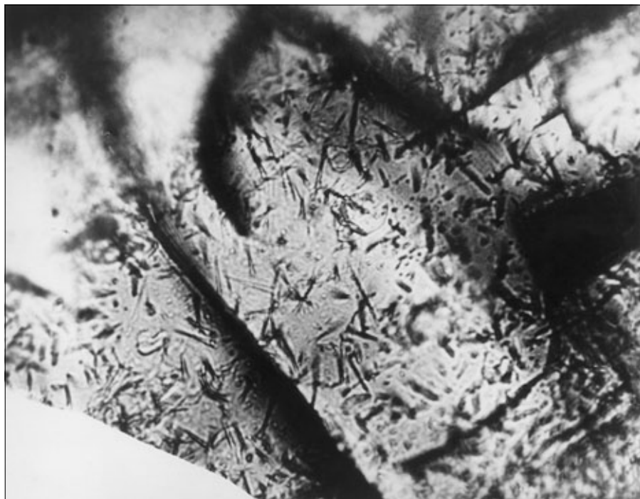
Figure 13.2. Tracks of cosmic rays, revealed after etching of a crystal from a lunar rock. Each of these tracks is less than 1/100 mm in length. (Photograph courtesy of Robert Walker, Washington University, St. Louis.)
