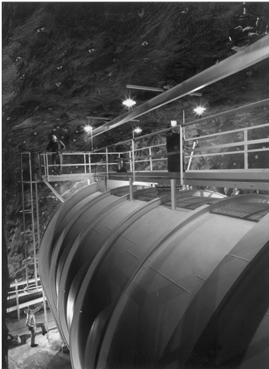
Figure 11.1. Tank containing 100,000 gallons of the neutrino detector perchlorethylene in the Homestake Gold Mine, South Dakota. (Photograph courtesy of Raymond Davis, Jr., and Brookhaven National Laboratory.)
