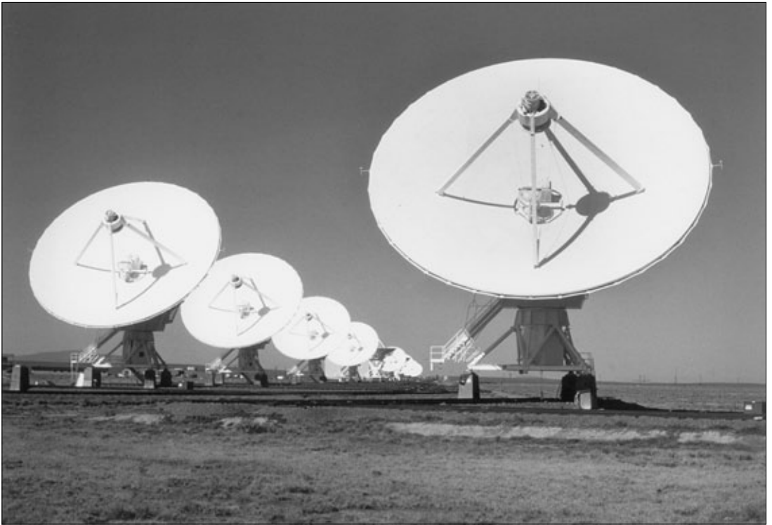
Figure 10.5. Modern radio antenna; 27 of these dishes can be moved on rails that extend along the three arms of the Very Large Array (VLA), located near Socorro, New Mexico. Each of the VLA arms is about 20 km long, and each dish has a diameter of 25 m. The spacing of the dishes can be changed, depending on the measurements that are to be made. (Photograph courtesy of NRAO/AUI.)
